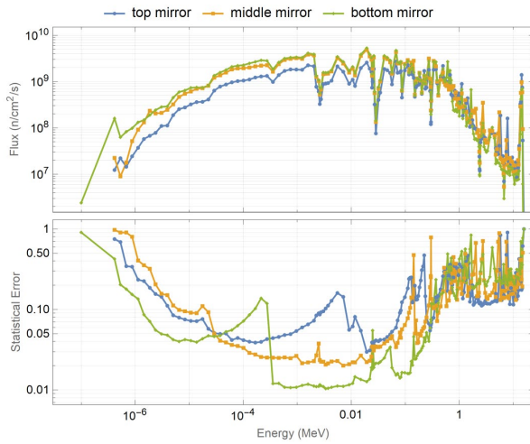
Figure 16: Neutron flux spectra ( \text{n/cm}^2/\text{s} ) in the first mirrors, for the 5-mirror configuration.
